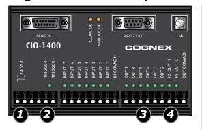
NOTE: The Trigger+ connector is wired to Input 0 on the Data-Man 100. The Triggerconnector is wired to Input Common while the unlabeled connector next to Trigger- is wired to Input 1 on the DataMan 100.
