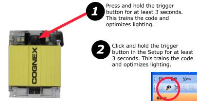
In the **Display** pane of the Setup Tool you can click the **Train Code** button to train the code, and you can click the **Optimize Lighting** button to optimize lighting.
