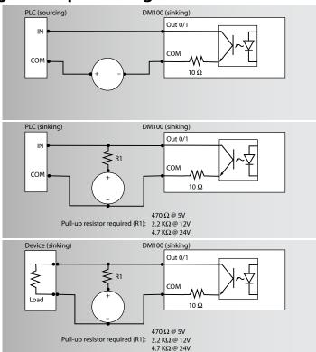
**Note:** These diagrams only apply to the Basic I/O module and to direct connections to the DataMan 100 input/output lines.
