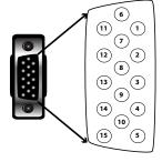
**Note:** Pin numbers are shown for cable connector, not I/O module.
